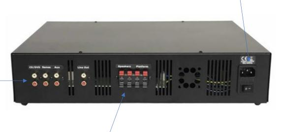
You need to connect the speaker wires colour to colour, so red to red and black to black. If a grayblack or wire is attached to the speakers, do gray on red and black on black. You also need to connect the speakers on the right side, so the left speaker on the left and the right speaker on the right. When used with a musical waterbed, it does not matter to the platform whether it is connected left or right.
