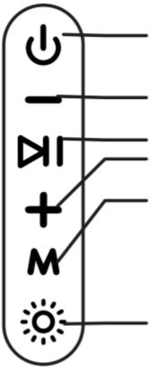
On/Off switch: Turn on. Press the switch for 3 seconds to turn off the device. If the device is not used for 30 minutes, it will automatically switch off.
