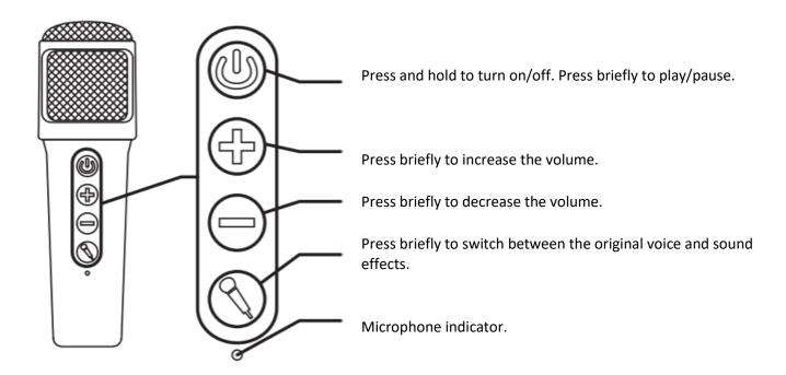
**Warning!** Do not forget to turn off the microphones before placing them in the dock to avoid the Larson effect.
