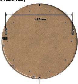
On the back of the panel you will find 2 hanging brackets. These are spaced 435 mm apart (centre to centre). Simply screw 2 screws into the desired mounting surface, at the correct distance, and hang the panel in place.
