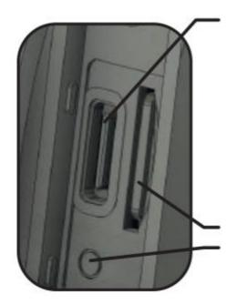
Charging port/USB-C connector DO NOT CHARGE THE BATTERY IF THE USB-C PORT IS WET. MAKE
