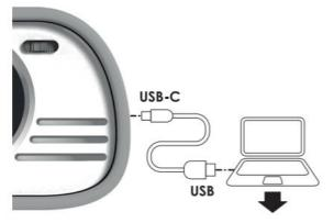
Turn on the KIDYCAM and connect the cable (USE THE ORIGINAL KIDYWOLF CABLE). Then check your computer.
