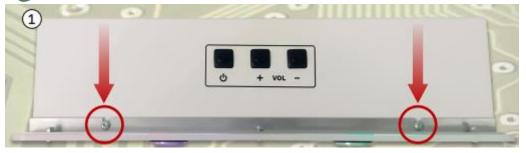
Once the screws have been loosened, the front Perspex face can be carefully hinged downwards (2). Do not let the door drop, as this can damage the Perspex front.
