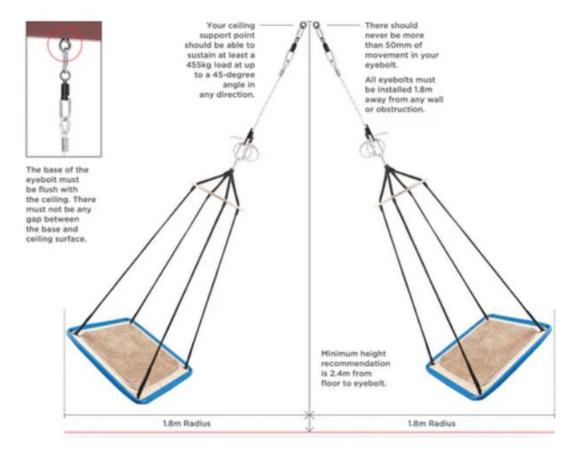
Movement of the eyebolt greater than 6.35 mm or any rotation under load is **UNSAFE**.
