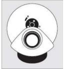
3. Install the included liquid wheel. This works with a magnetic adapter - the slider on the left side of the magnetic adapter should be at the top , as shown in the image. Place the magnetic wheel on the magnetic adapter on the projector. To remove the wheel, you can lift the wheel.
