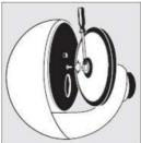
After removing the magnetic adapter, push the wheel onto the axle of the wheel motor, as shown. This is easier if you turn the effect wheel lightly, with up and down movements.
