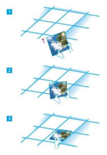
See the layout for the correct placement. Directional arrows and digits are placed on the back of the panel and on the layout. Watch out not to touch the panel on the image and in the middle. Only touch the aluminum frame to prevent fingerprints and light openings.
