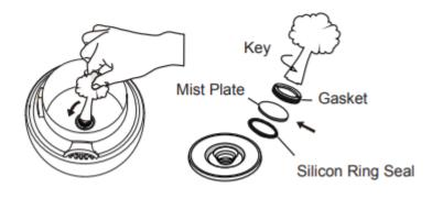
Follow the diagram, remove the original Mist Plate by unscrewing the Gasket using the Key provided. Replace a new Mist Plate and press tightly onto the Silicon ring seal. Screw back the Gasket with the Key to secure
